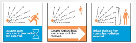
The less **TIME** spent near radioactive material, the less dose received.
