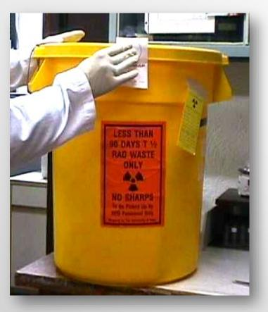
Wipe test the entire external surface of the container.
