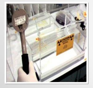
**To perform a meter survey** slowly pass the probe over the area or object to be surveyed. Move the probe at about 2 cm per second.
