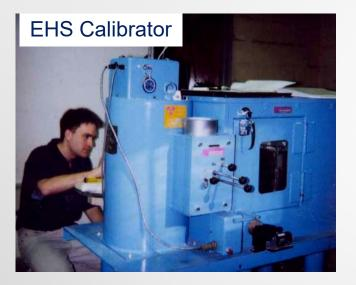
Survey instruments used for contamination and exposure rate surveys must be calibrated every 12 months.
