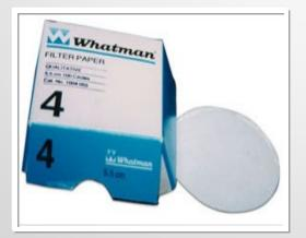
To conduct a wipe survey, all you need is a piece of filter paper or a paper towel cut into  $1.5'' \times 1.5''$  strips.
