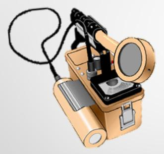
Survey meters are used to measure radiation absorbed dose.
